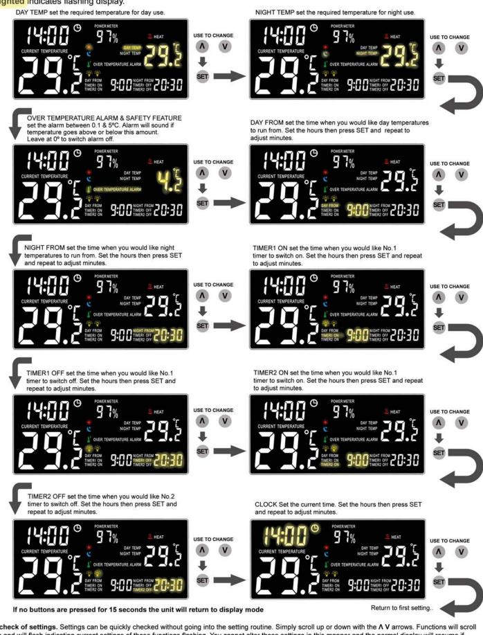
Quick check of settings. Settings can be quickly checked without going into the setting routine. Simply scroll up or down with the A V arrows. Functions will scroll through and will flash indicating current settings of those functions flashing. You cannot alter these settings in this manner and the normal display will resume if
